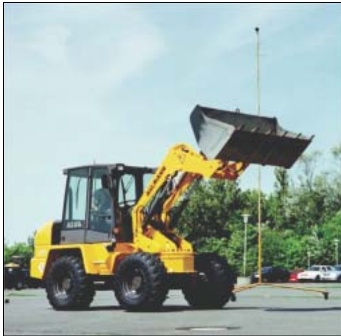
Fig. 2 Olaf Klomfass and the AZ85t loader in action. Notice the Ahlmann-designed 11 m high microphone stand that is easily erected at the test site
