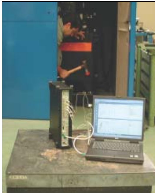
Fig. 3 Jon Irazusta is the sound and vibration technician at AMC. Here he is using an impact hammer to check the vibration response of a damper
