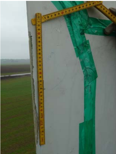
Fig. 11. Implementation of artificial blade damage - extended to 30 cm (left); extended to 45 cm (right)
