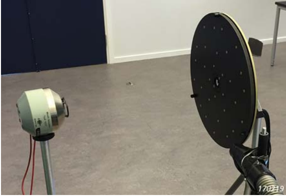
Fig. 7. Picture of the setup with the array (right), sound source (left) and flow-beam hose (bottom right)
