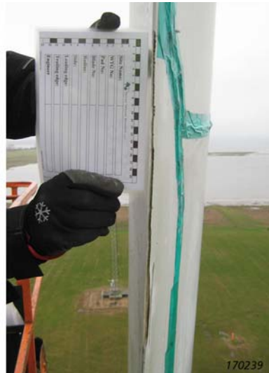
Fig. 11. Implementation of artificial blade damage - extended to 30 cm (left); extended to 45 cm (right)
