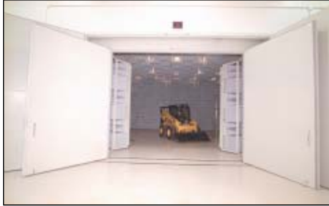
Fig. 5 The chamber is large enough for complete machines to be tested
